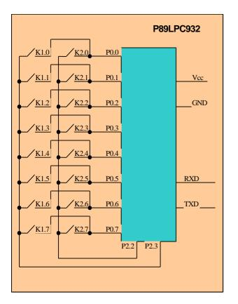
registers are: the Keypad Interrupt Mask Register (KBMASK), the Keypad Pattern Register (KBPATN) and the Keypad Interrupt Control Register (KBCON). The first register (KBMASK) is used to define which input pin connected to Port 0 is enabled to generate
